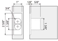
Chisel a 1 /8" deep indentation within the traces of the strike. Place the strike flush with the door frame and secure it with screws.
